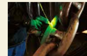
Magnetic particle inspection.
